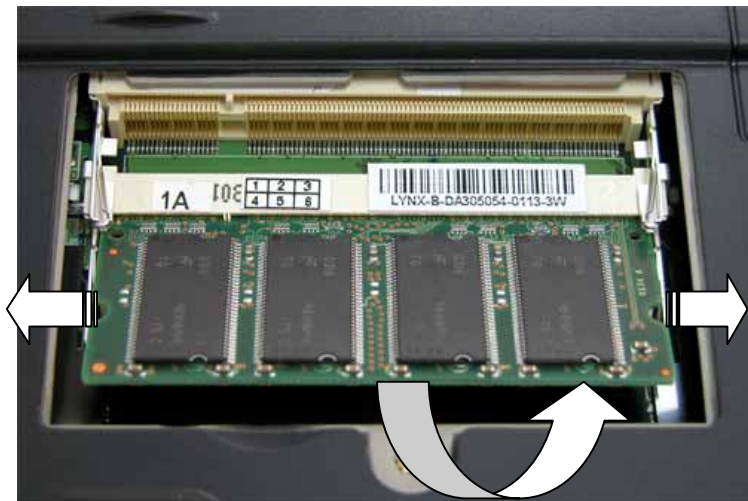
Fig. 7 Removing the memory module
